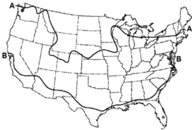
Figure 14–9. A, the northern limit of recorded damage done by subterranean termites in the United States; B, the northern limit of damage done by dry-wood termites.
