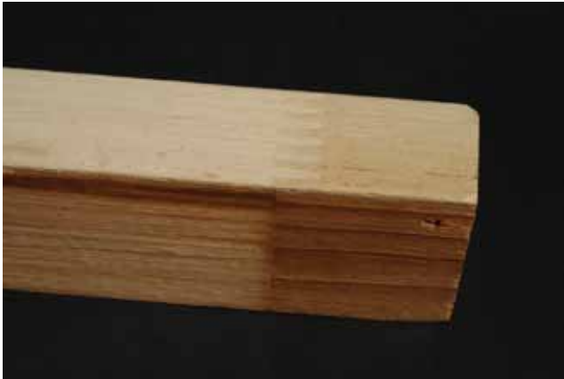
Figure 16-10. Differences in stain from extractives on fingerjointed wood from the white pine group (either eastern or western species) painted with acrylic solid-color stain.
