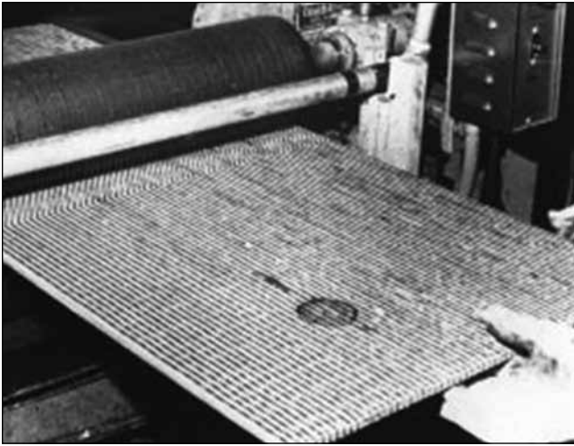
Figure 10–6. An extruder applies continuous and uniformly sized and spaced beads of adhesive to veneer for laminating into laminated veneer lumber (LVL).
