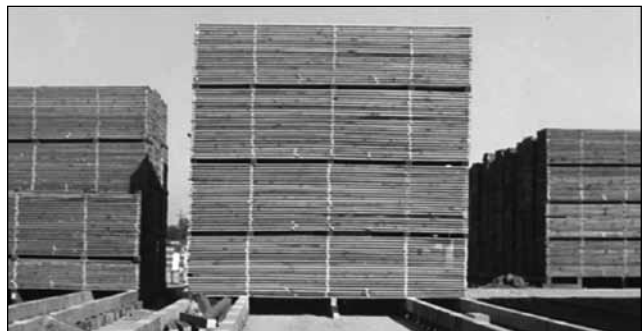
Figure 14-7. A sanitary, well-drained air-drying yard.
