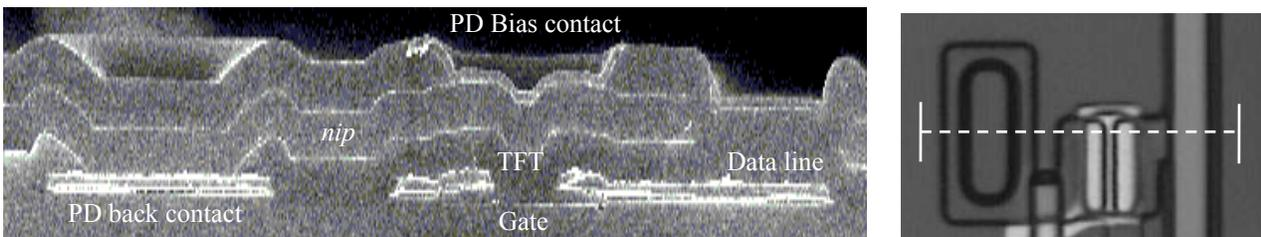
**Figure 3.** (a) SEM cross-section of the MF pixel. (b) Line across pixel where the cross-section was made.
