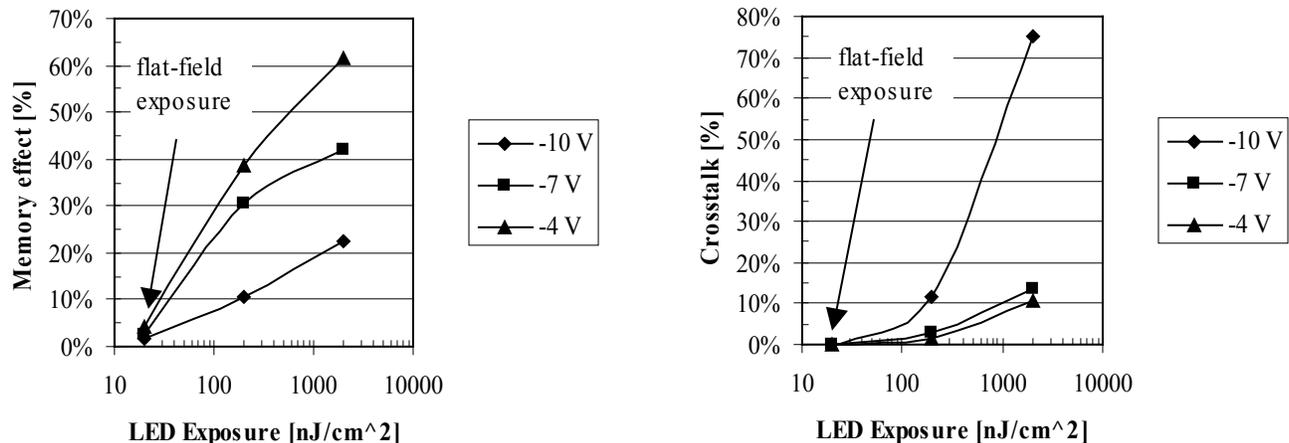
**Figure 7.** The memory effect and crosstalk as a function of LED exposure and array bias.
