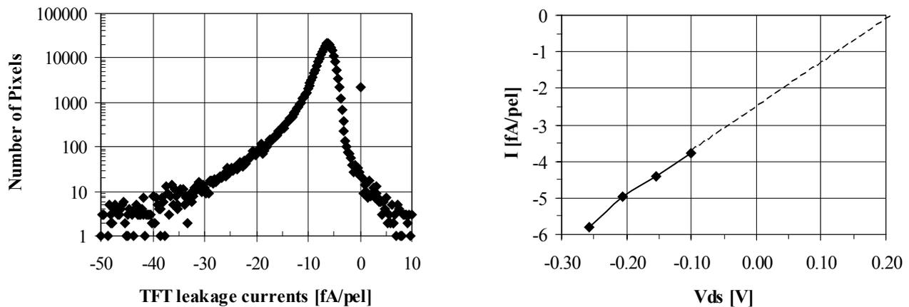
**Figure 12.** (a) Histogram of TFT leakage currents at 967 $\mu\text{R}/\text{frame}$ .
