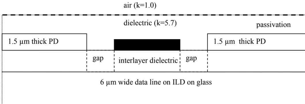
**Figure 8.** The top of each photodiode (PD) is held at constant bias potential; the bottom of each photodiode forms a floating collection electrode which is strongly coupled to bias potential through the capacitance of each photodiode.
