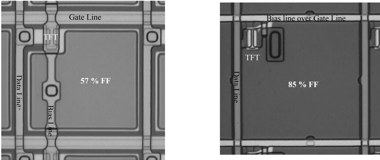
**Figure 1.** Comparison between 57% FF baseline and 85% FF MaxFill™ 127 μm pixel designs.
