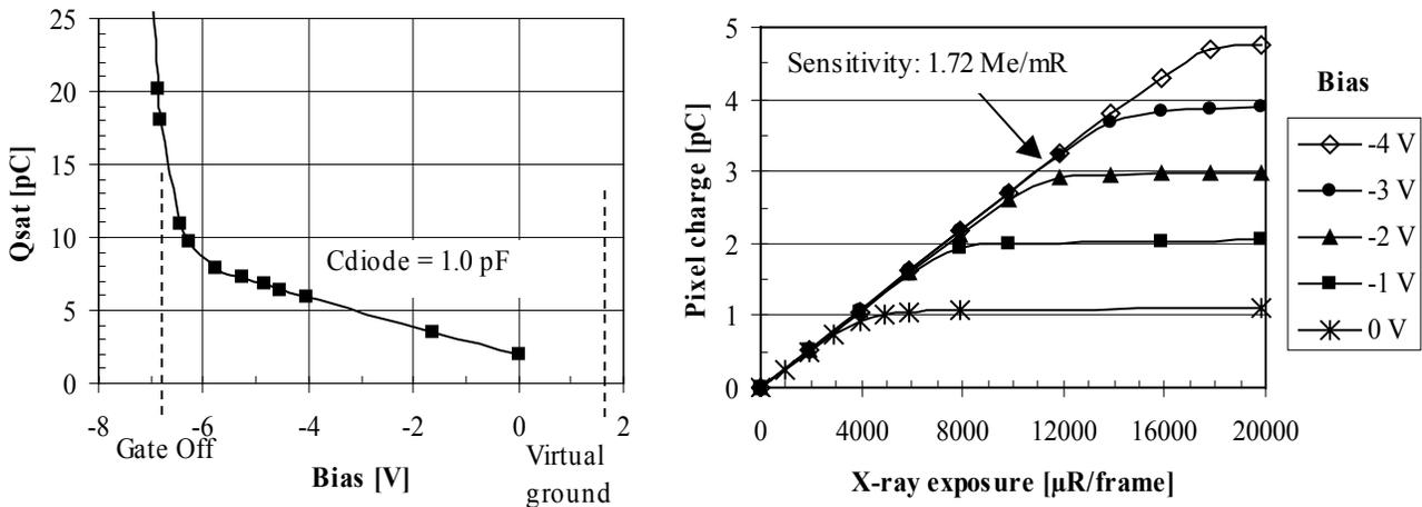
**Figure 10.** (a) Saturation charge measured vs. bias.
