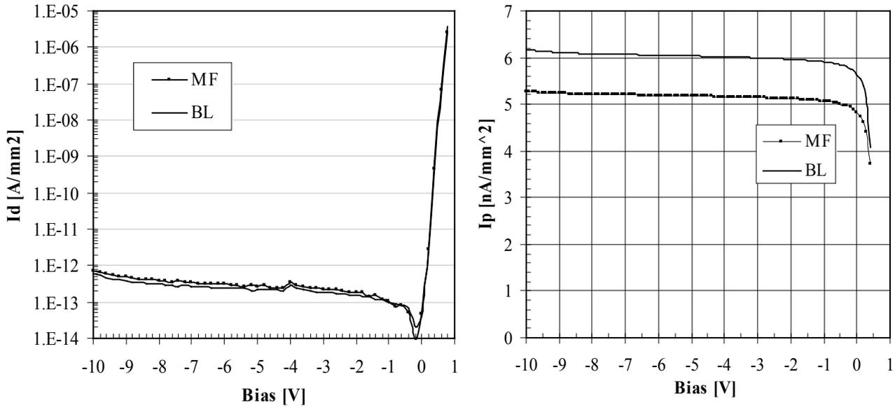
Figure 4. (a)  $I_d(V)$  for BL and MF photodiodes in the dark.
