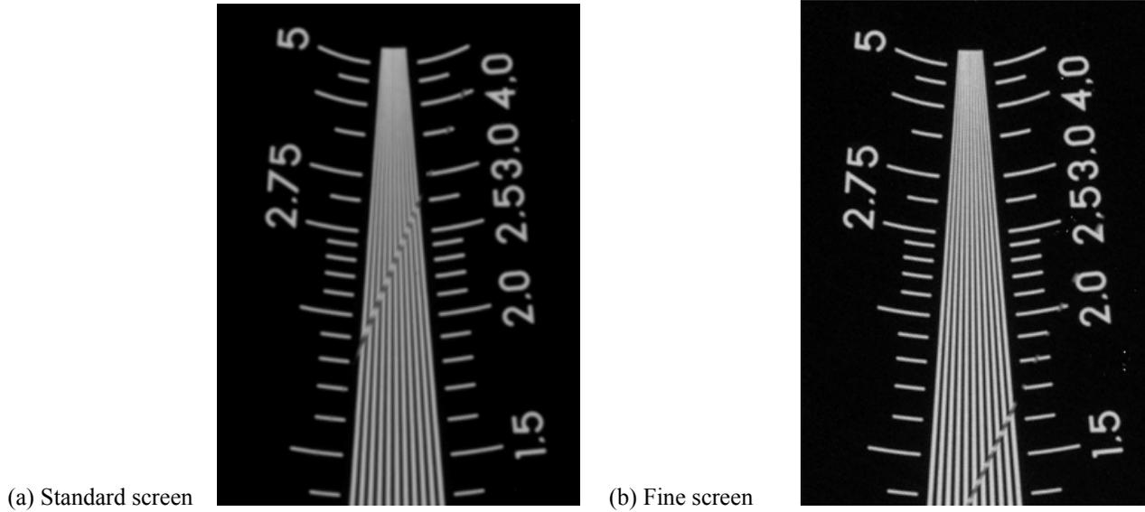
**Figure 13.** Images taken from the detector with (a) the standard screen, and (b) a fine screen. The line-pair patterns are fully resolved out to the Nyquist limit of 3.94 LP/mm in both cases, although the resolution is much better with the fine screen.
