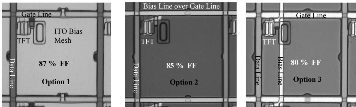
**Figure 2.** Different connection schemes for connecting bias to each photodiode: Option 1: ITO bias mesh; Option 2: bias line running over gate line; and Option 3: bias line running parallel to data line.
