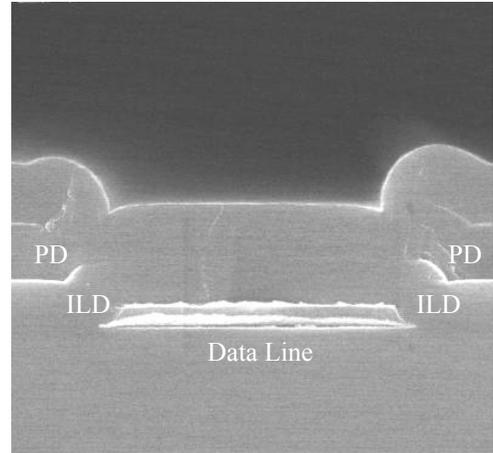
**Figure 9.** (a) Data line to bias capacitance as a function of gap between the data line and photodiodes, modeled with FastCap and measured on test arrays of 127  $\mu\text{m}$  pixels. (b) SEM cross-section of photodiodes and ILD near a data line.
