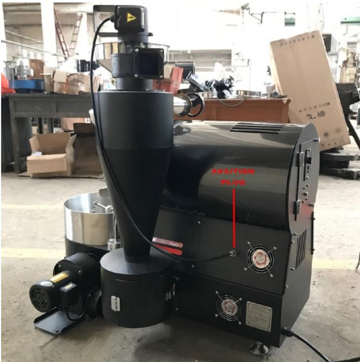
**IMPORTANT:** Always connect aviation plug to roaster while unit is unplugged. Never attach or remove aviation plug when unit is plugged in or machine is on.
