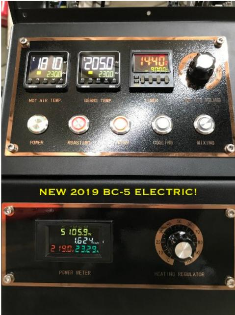
**NEW FOR 2019: POWER METER:** SHOWS THE WATTAGE, VOLTAGE AND AMPS BEING USED AT ANY GIVEN TIME. **(PANEL LIGHTS UP WHEN TURNING THE HEATING REGULATOR UP)**
