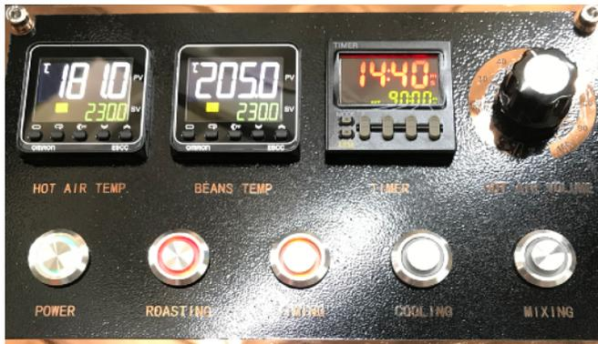
**TWO OMRON TEMPERATURE CONTROLS FOR BT & ET ONE TIMER FOR TIMING ROASTS (RESET BUTTON ON LEFT BOTTOM)**
