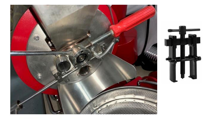
ONCE REMOVED YOU WILL NEED TO REMOVE OLD BEARING FROM THE CASING:
