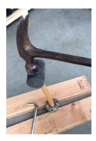
NEXT YOU WILL WANT TO PUT NEW BEARING INTO CASING. YOU MAY NEED LUBRICANT OR HEAT TO SEAT NEW BEARING INTO HOLDER. ONCE DONE REASSEMBLE UNIT: YOU MAY NEED TO PUSH UP ON BEARING HOLDER TO GET IT IN PLACE TO PUT BOLTS ON: ONCE ALL BOLT AND COVERS ARE IN TIGHTEN AND TEST
