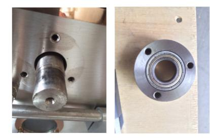
ONE WAY TO REMOVE BEARING FROM CASING IS TO SET IT BETWEEN A COUPLE 2x4'S AND USING A WOOD HANDLE OR DOWEL YOU CAN TAP ON DOWEL TO REMOVE OLD BEARING
