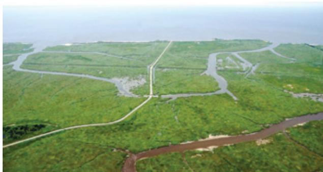
**TORN SALT MARSH** in Delaware Bay (*top, 1998*) was restored by cutting a few gaps in adjacent dikes so freshwater could flow in and naturally create tidal creeks, which allowed plants to reseed and flourish (*bottom, 2013*).
