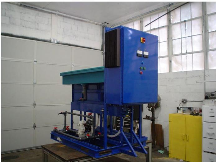
15 gpm Electrocoagulation Unit
