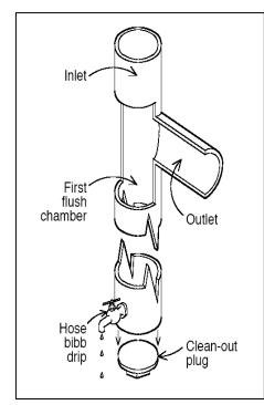
Figure 2-2. Standpipe first-flush diverter
