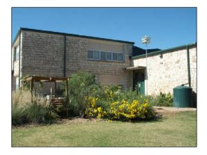
Menard Elementary School rainwater harvesting installation showing downspout, 1,000-gallon poly tank, and gazebo (left) surrounded by native and adapted landscape plants. In this very attractive installation, harvested rainwater (using existing gutter and downspouts) furnishes water not only to the landscape, but also to a watering pond, birdbath, and wildlife guzzler. (Photo courtesy: Billy Kniffen)
