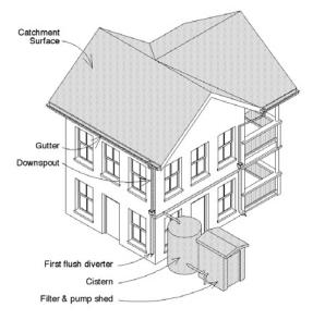
Figure 2-1. Typical rainwater harvesting installation
