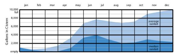
Figure 4-4. Volume of water in storage, using average rainfall data and median rainfall data for Dallas, Texas
