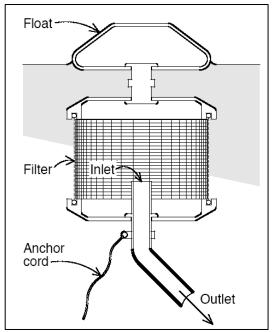
Figure 2-11. Cistern float filter
