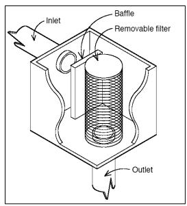
Figure 2-4. Box roof washer
