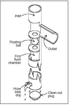
Figure 2-3. Standpipe with ball valve
