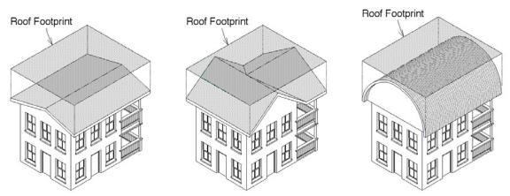
Figure 4-1. Catchment areas of three different roofs
