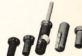
BHT4 —Famous Black Hawk Tapering Tool. This tool acclaimed by all as the finest tapering tool on the market, designed to fit all points and nocks. Included are four bushings which have tapered sleeves that fit in a tapered hole of the main tool. Bushings are 1/4", 9/32," 5/16," and 11/32" and are slightly oversized to permit clearance of oversized shafts or painted shafts. Blade for cutting is a used injector-type razor blade, available at any drug store. (Directions and descriptive literature with each tool.) Complete tool containing six parts.
