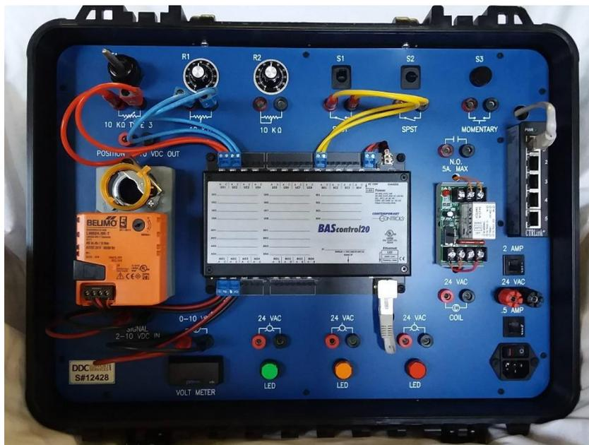
has a built-in handle and a removable cover. The case can be permanently mounted to a tabletop using the integral mounting slots. A variety of banana plug jumper cables are included for controller wiring. A
