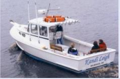
The Kandi Leigh is a 28' lobster style boat built in Jonesport Maine. A classic cedar over oak design the boat has been meticulously maintained and cleaned. Although traditional in style the boat is equipped with all the Coast Guard safety equipment and modern electronics including: VHF radio, cell phone, radar, & GPS. There is a fully functional head aboard the boat as well.
