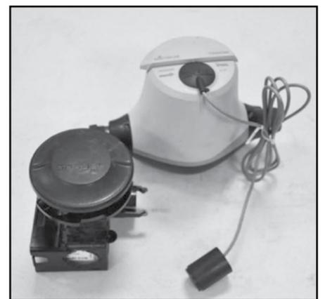
The new AMI transmitter assembly will be applied to new water meters that are equipped to call in their own readings.
