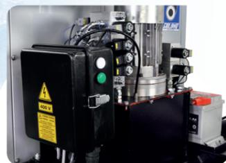
Electro-hydraulic unit with easy inspection area, for fast checking and maintenance.
