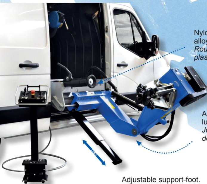
Nylon bead breaker Roller for alloy wheels.
