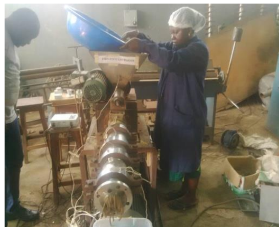
Figure 2. Showing extrusion of the extrudates
