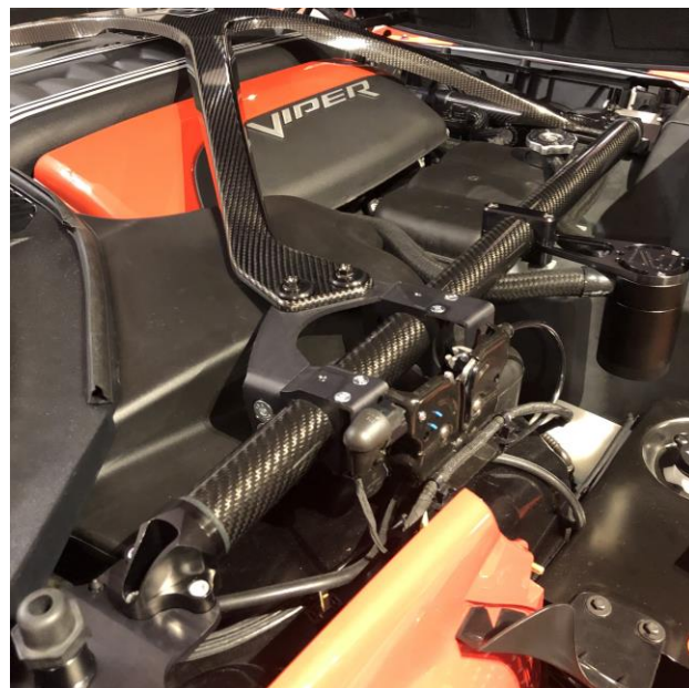
Passenger Side Lateral Carbon Fiber Engine Brace Installed
