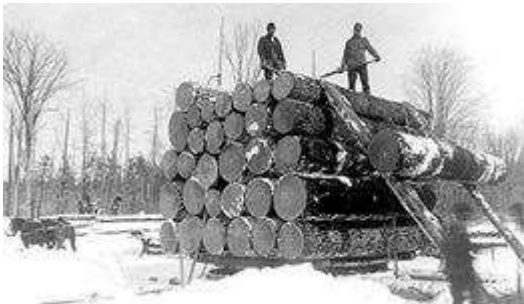
Stacking was done with a system of chains loaded from the side with other horses. Chains reattached at every tier to pull the logs higher. Logging was and is yet a very dangerous and demanding occupation. This White Pine from Northern Michigan was logged off to rebuild Chicago.
