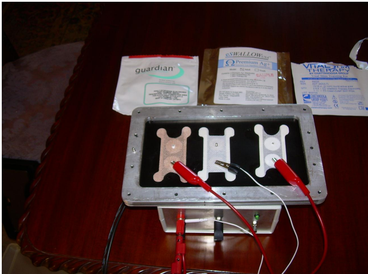
Figure 1. Picture of the Dispersion Test setup.
