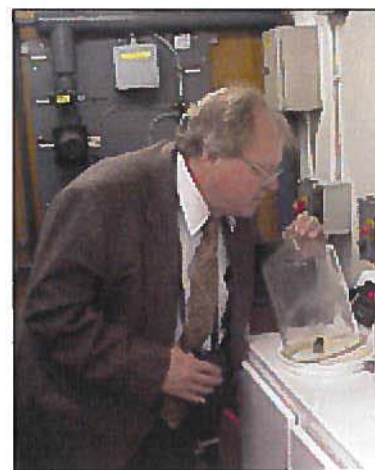
The "smell bell" test is being performed here on a sample from the River Trent in the United Kingdom. The smell bell test is an inexpensive method of physical analysis but requires trained personnel with good noses and usually is not performed more than once per shift or once per day.
