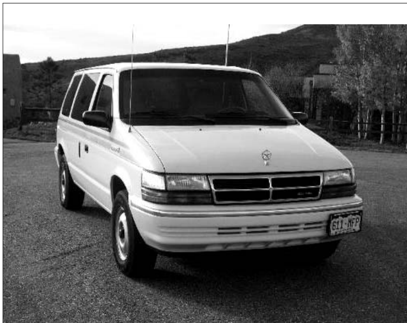
A Chrysler TEVan, used as a test bed for the Ovonic battery pack
