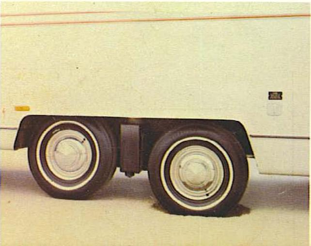
Avion builds strength from the bottom up. Our triple-beam frame of heavy-duty steel is five inches deep on 25 and 28 foot trailers, and six inches deep on 31 foot models. Bolted to the frame is a 2 $\frac{3}{8}$  inch insulated floor.
