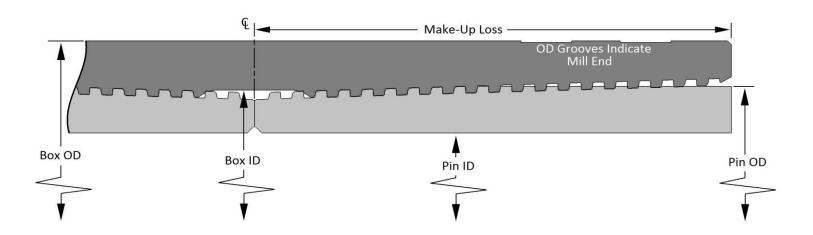
$<sup>^{2\</sup>cdot}$  If Optimum Torque does not meet the Base of Triangle Stamp, M/U to the Base of Triangle.
