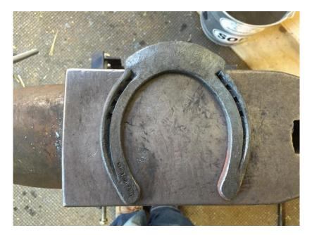
These are handmade steel shoes with a toe extension made specifically for this case. Frequently with therapeutic cases it is necessary for a farrier to hand make a custom shoe.
