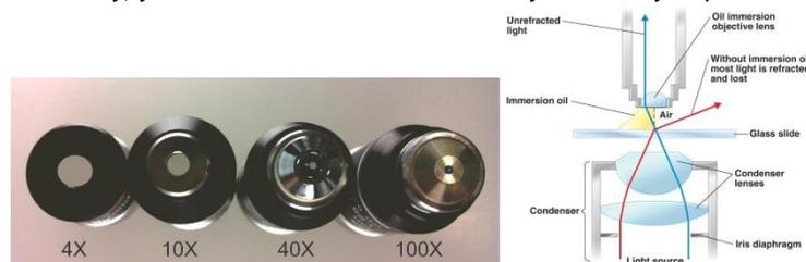
Figure 3: Photograph of the four objective lenses of the Nikon Alphaphot-2. Note the decreasing size of the objective hole as the magnification increases.
