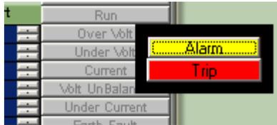
Alarm is active immediately when the level exceeds the voltage unbalance setting. Trip is active when the level exceeds the voltage unbalance setting and after the definite time delay expired. If latch on last trip is selected the output will stay active until the M20E has been reset.
