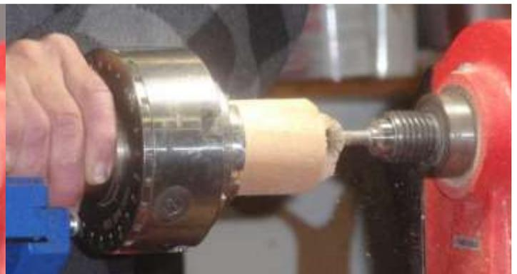
Ian is in the midst of cutting exterior threads on the top of the box to accept the lid.
