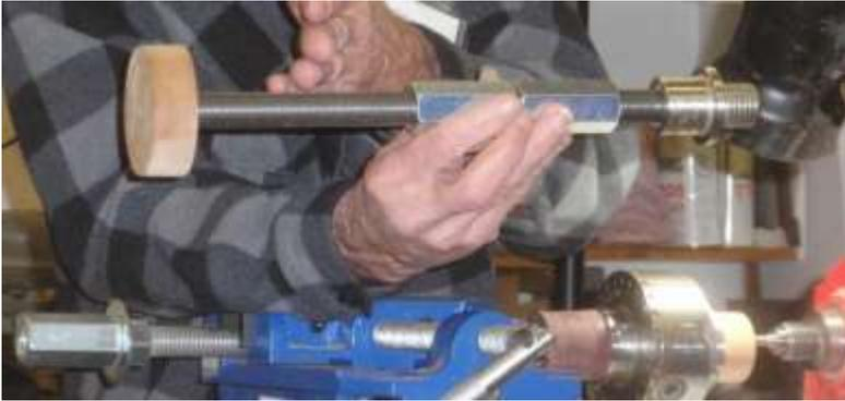
Here is the jig with the collet chuck at the end ready to accept the larger chuck.
