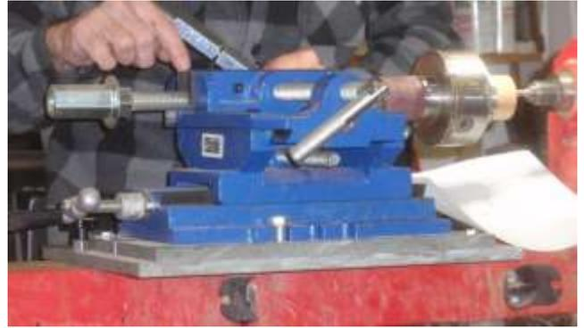
Pictured is the slide Ian purchased from Harbor Freight for around \$60. It holds the jig (from photo #2) which has been fitted with a Purpleheart adapter/ spacer for the chuck. It is positioned close to the headstock with the cutter engaged in cutting the inside thread of the lid.
