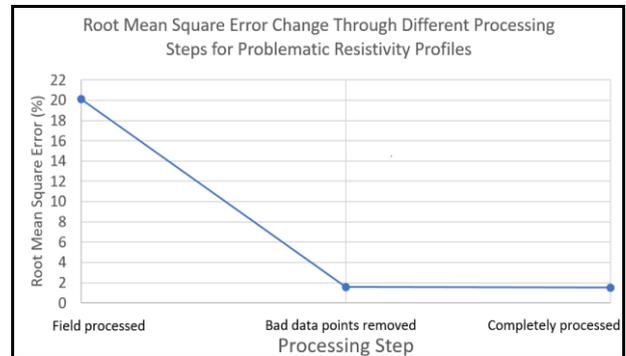
Figure 3. Root mean square (RMS) error change through different processing steps. Up to a 20 % reduction in RMS error is achieved in some of the resistivity profiles. This reduces the error in apparent resistivity contours from ± 235.57 Ω·m to ± 15.86 Ω·m. The improvement in RMS error shifts the resistivity contours and the geological model layers to the correct depths.
