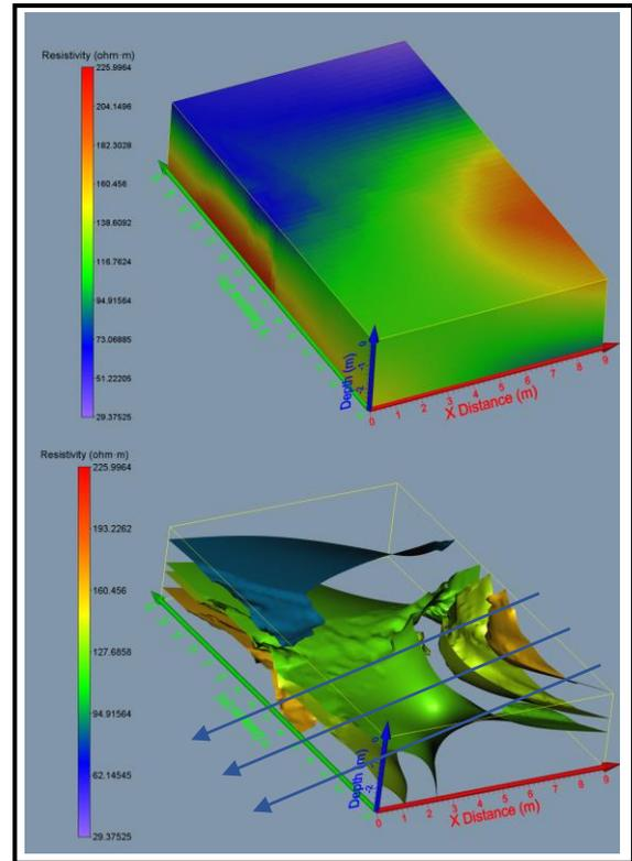
**Figure 6.** Surface render of 3DRA1 (top) and isosurface plot of 3DRA1 (bottom). Blue arrows indicate possible water flow path.
