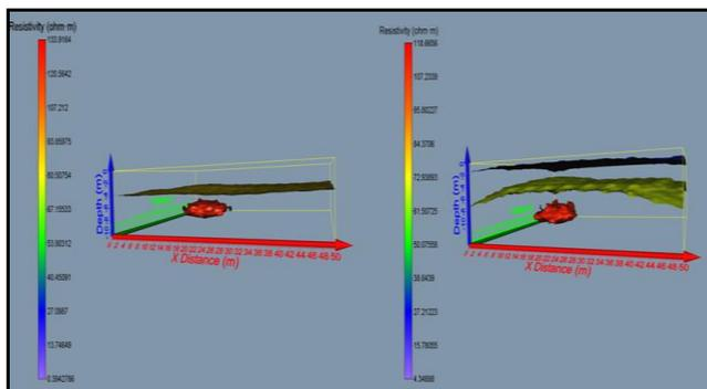
**Figure 8.** Wenner-Schlumberger (left) and dipole-dipole (right) Synthetic boulder three dimensional resistivity model. The red shape is the detected boulder within the model.
