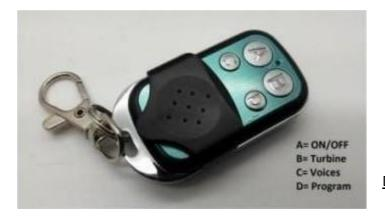
Press "A" 1 time = on/off scanner (<u>if REM is disconnected</u>)
