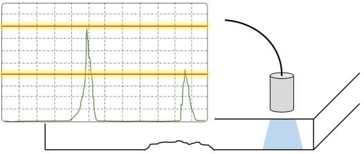
Set the first back-wall at 80% full screen height. This is assuming that the unit is in the standard mode, not echo-to-echo mode. Echo-to-echo is another article for another day.
