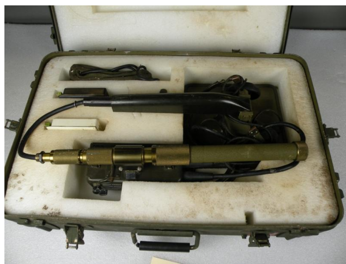
The AN/PRS-7 is the rarest of all the Army mine detectors. Most of the AN/PRS-7s were upgraded to AN/PRS-8s. The two detectors shared the same housings, but the AN/PRS-8 had upgraded electronics. The only visible way to tell the difference between the two detectors is by the data plate.
