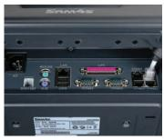
*Easy to Access Ports* Connect to a wide array of compatible off-the-shelf POS peripherals with six serial ports and two USB ports.
