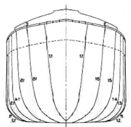
Figure 5. Full-width template of the bow portion.
