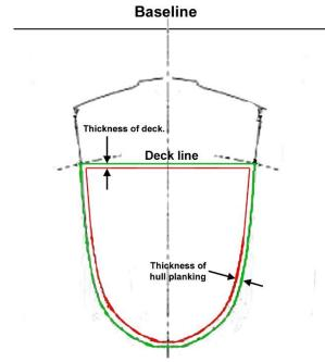
Figure 8. The rib outline modified for deck and planking thickness. The outer line is the original outline from the Body Plan; the inner line shows the shape required inside the hull.
