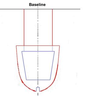
Figure 12. Finished outline of rib 16 template – as prepared for internal hull access - with vertical cuts to remove extension.
