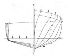
Figure 19. A section through a hull of mixed type.
