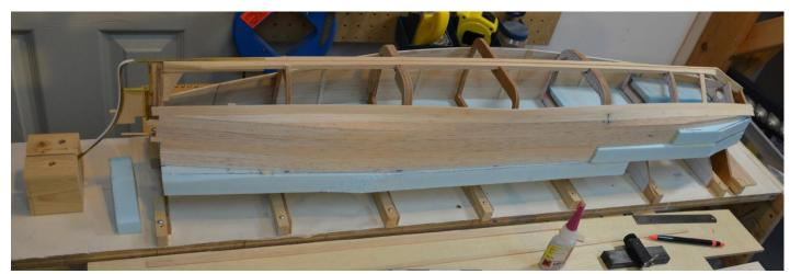
Figure 18. Roy's *Wahine* hull during planking. On this hull, blue foam insulation was used along the top edge of the hull, and planking started from there.
