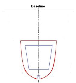
Figure 10. Rib 16 showing in blue the internal cutout and the notch for the keel.
