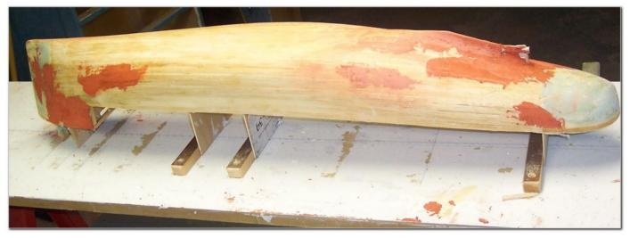
Figure 21. Radley's (Steve M's dad) trawler hull after shaping of the bow and stern, removal of some of the rib extensions, and with Bondo applied. Ready for painting.
