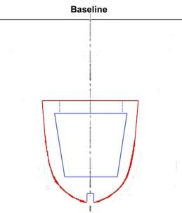
Figure 11. Cutting lines added to top part of rib.
