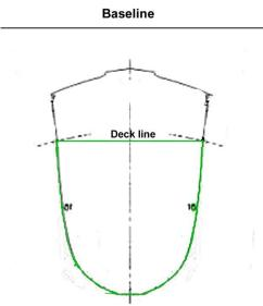
Figure 7. The basic outline of rib 16 from the Body Plan.
