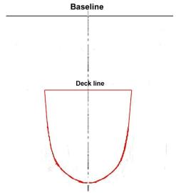
Figure 9. The internal outline of the hull at rib 16.
