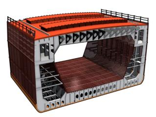
Figure 2. Section through a ship's hull.
