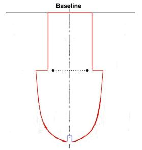
Figure 13. Making a horizontal cut to remove the extension.
