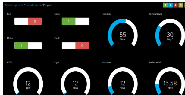
Fig. 5: Adafruit server to see relay condition and sensor readings
