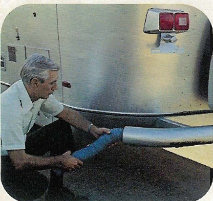
Rear bumper stores flexible tube for draining waste and sewage tanks
