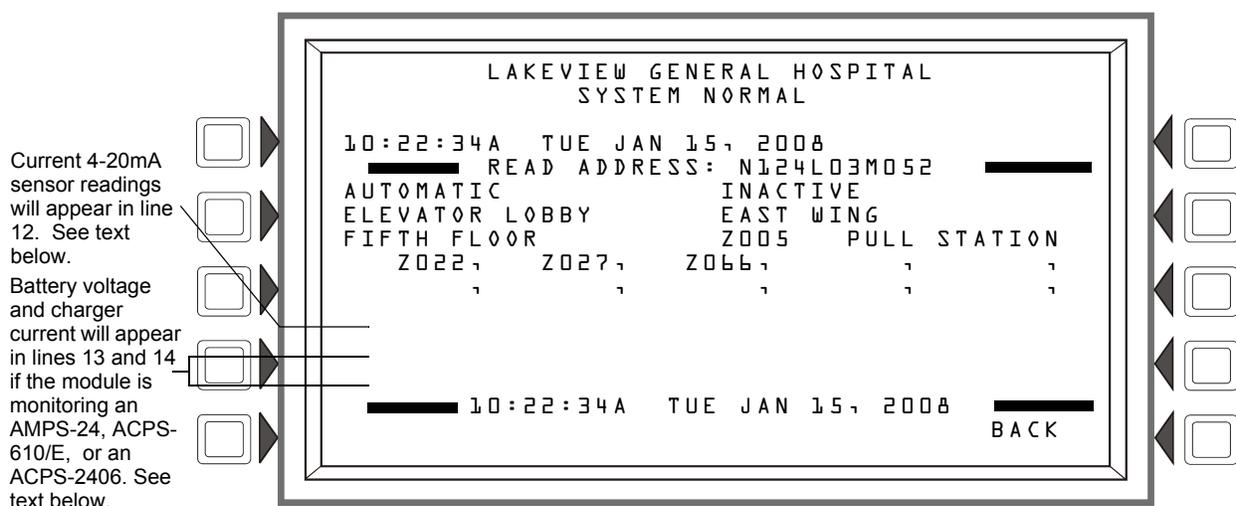
**Figure 3.4 Monitor Module Screen - Read Status**
