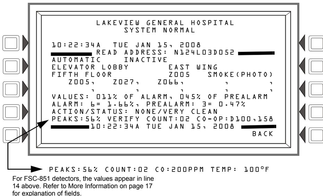
**Figure 3.2 Smoke Detector Screen - Read Status**
