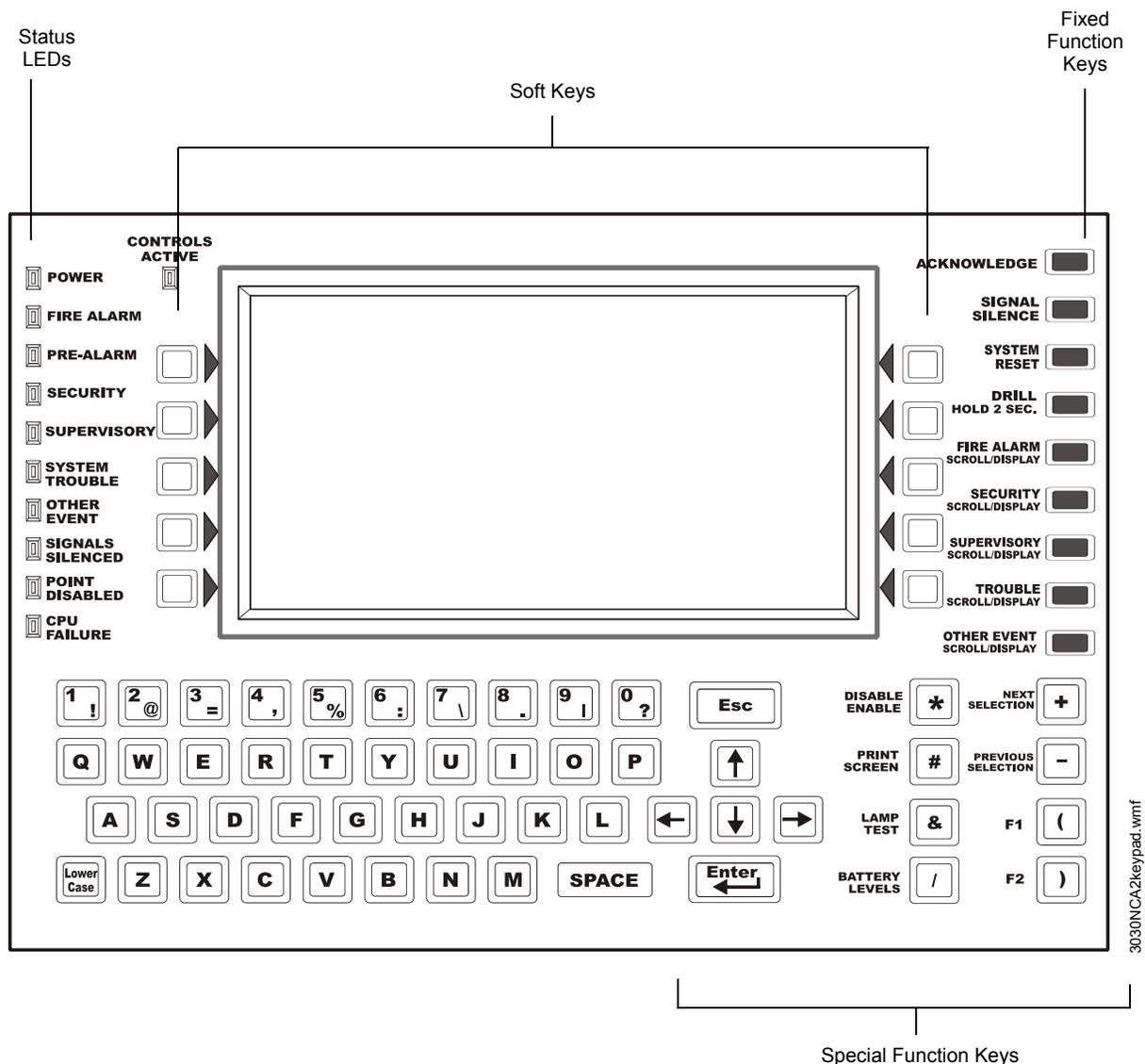
Figure 1.1 The Display/Keypad
