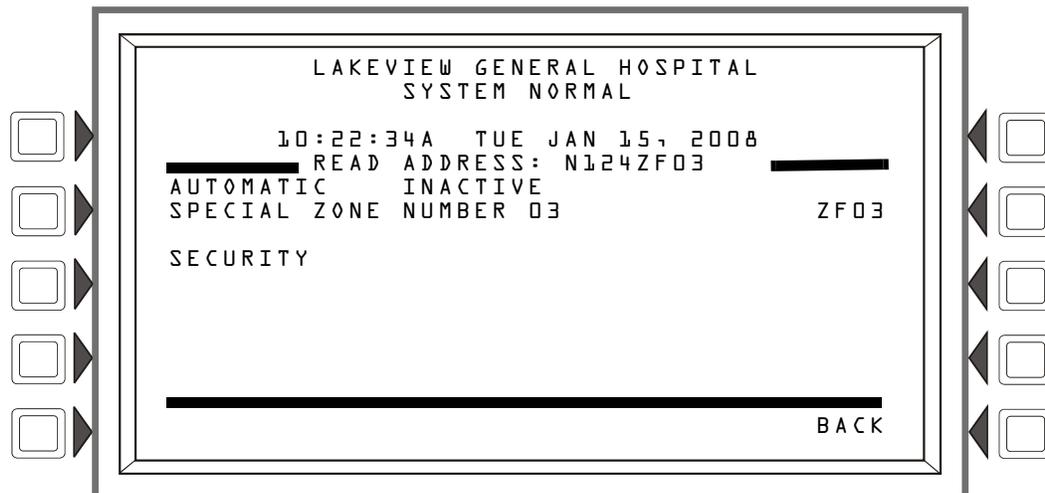
**Figure 3.9 Special Function Zone Screen - Read Status**
