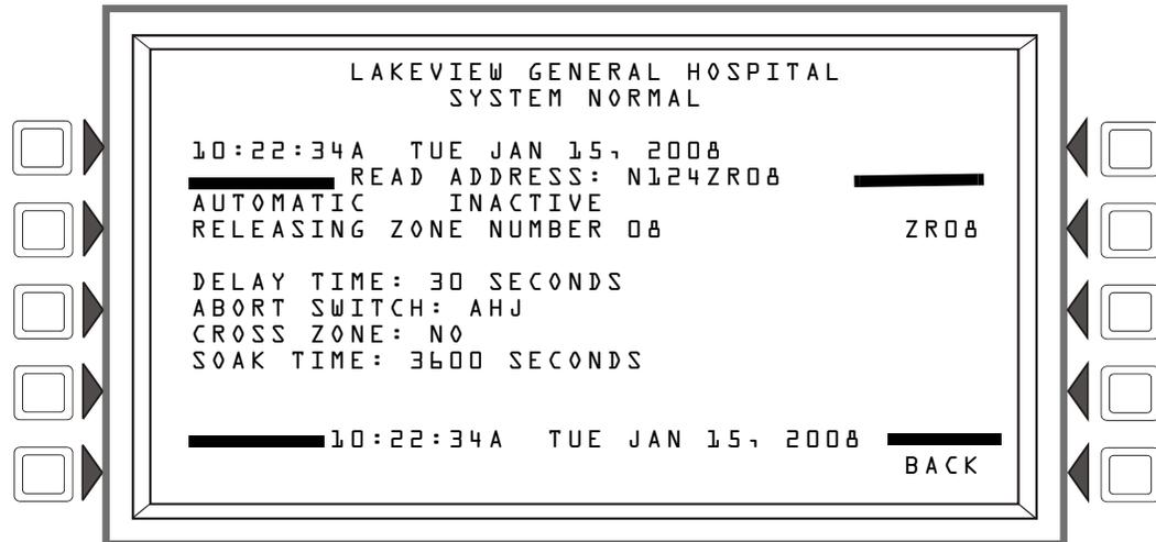
**Figure 3.8 Releasing Zone Screen - Read Status**
