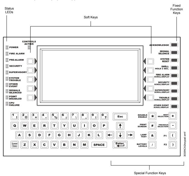
Figure 1.1 The Display/Keypad
