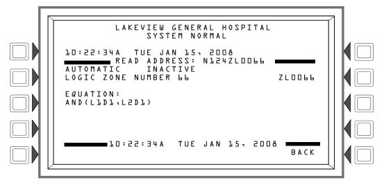
Figure 3.7 Logic Zone Screen - Read Status
