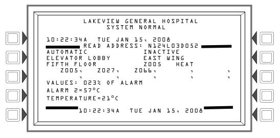
Figure 3.3 Heat Detector Screen - Read Status
