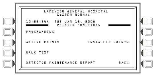
Figure 5.1 Printer Functions Screen
