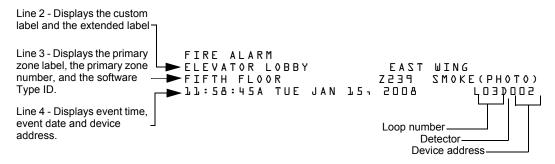
The point event example screen below shows a trouble condition that has been generated by the detector on loop 3, address 2.
