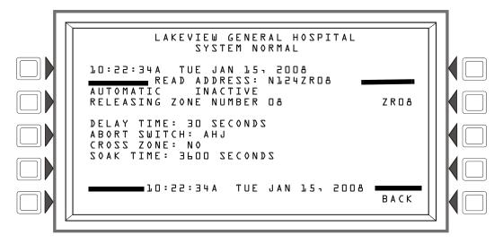
Figure 3.8 Releasing Zone Screen - Read Status
