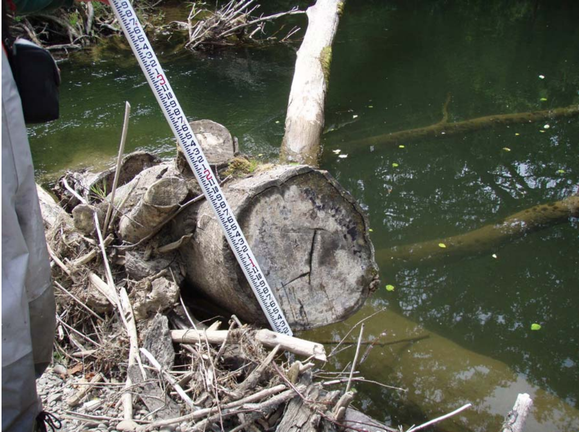
Figure 3.17. Photograph showing that LWD in jam photograph above was cut in place.
