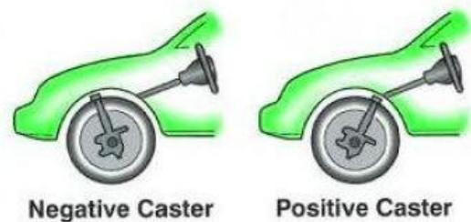
Figure 1.5: Wheel Alignment.
