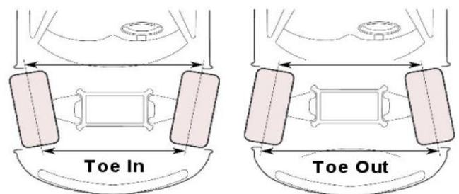
Figure 1.1: Toe Measurement.
