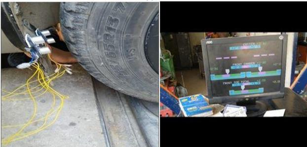
Figure 1.8: Target for Detection of Wheel Alignment.
