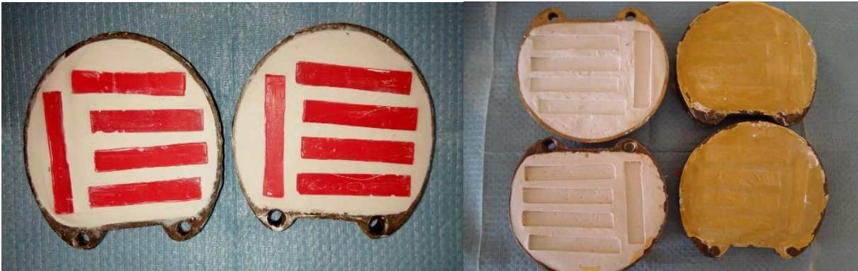
Fig 2: Standard dies were flasked to obtain mould space for acrylic specimen preparation
