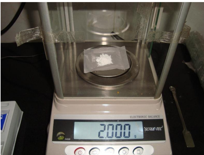
Fig 4: Sensitive balance having sensitivity of 0.001gm and capacity of 10 gms
