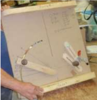
Lenny Mandeville showed his segmenting sled and lathe drum sander jig. He got information on how to build them from Stephen Ogle's Youtube video's – (example is : https://www.youtube.com/watch?v=-XWzyLe6bsQ )
