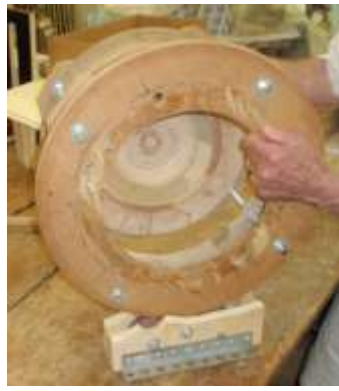
You are looking at two views of Wally's sandwich chuck that adjusts to hold spheres for being hollowed out. The middle picture also shows the "steady rest that Wally made to support the weight of the sandwich chuck.
