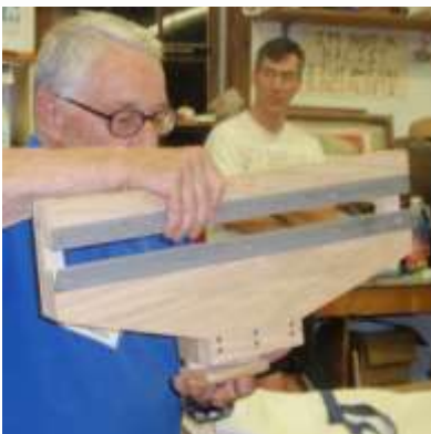
Ben had a large burl to hollow so he went to see Wally and copied this toolrest to hold his hollowing tool ala Jamison style. Ben made a routing jig (3 rd picture) to cut grooves lengthwise on a vase as seen in the photo that he holds (second from the left). The 4th picture shows his Dremel and routing jig that he used. The Dremel router traveled in the metal groove shown in the 3 rd picture.
