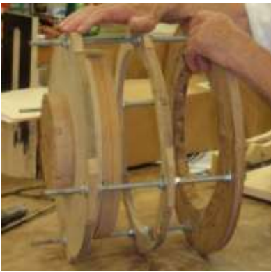
You are looking at two views of Wally's sandwich chuck that adjusts to hold spheres for being hollowed out. The middle picture also shows the "steady rest that Wally made to support the weight of the sandwich chuck.
