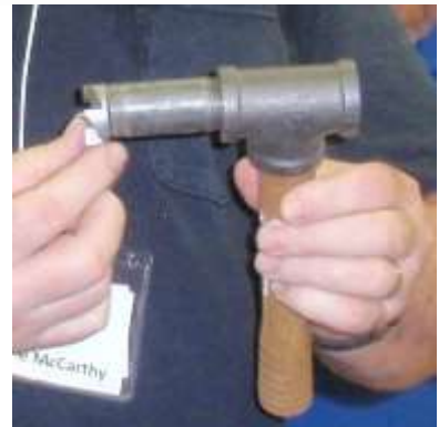
Charlie McCarthy holds a hammer constructed from a pipe fitting attached to a handle that he uses to pound a four prong spur drive into a blank without damaging the spur drive.
