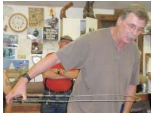
Nigel holds a measuring device he welded together to use for determining the thickness of a deep hollow form, or other closed vessel, when hollowing out the inside
