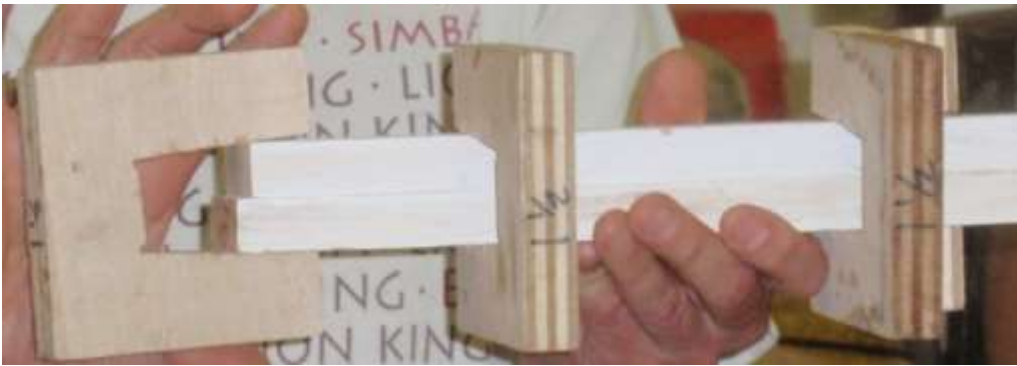
Mike Veno showed us his specially made clamps for holding two pieces of wood together when glued for drying. If you have several same thickness pieces, this is a real time saver.
