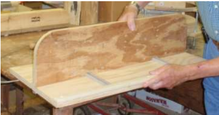
Ron Reynolds showed a sled for use with his Bandsaw which he uses to cut thin pieces with.
