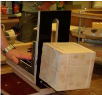
Wayne Miller showed us his wave box. The cut in the bowl is made by using swivels to set the radius to allow for the curve of for straight cuts. You bend the wood after steaming in the microwave. Then the steamed wood can be glued to the form.
