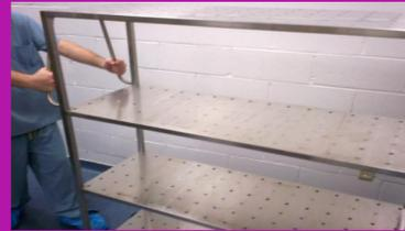
**Figure 2.** To minimize hand contusion injuries, we modified shelving units by installing ergonomic handles, with sufficient margin from the exterior edges of the equipment.
