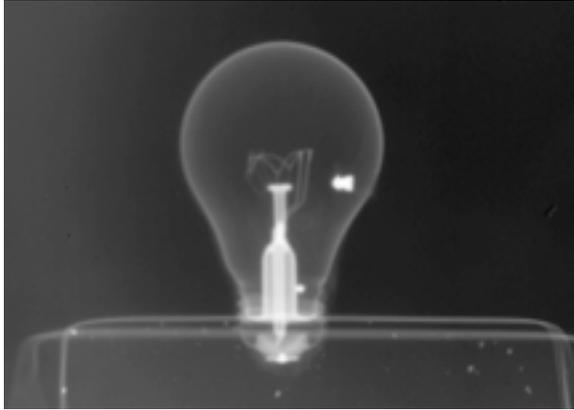
Figure 12: A digital x-ray of a bullet fired into a light bulb, taken with a fast x-ray pulse.
