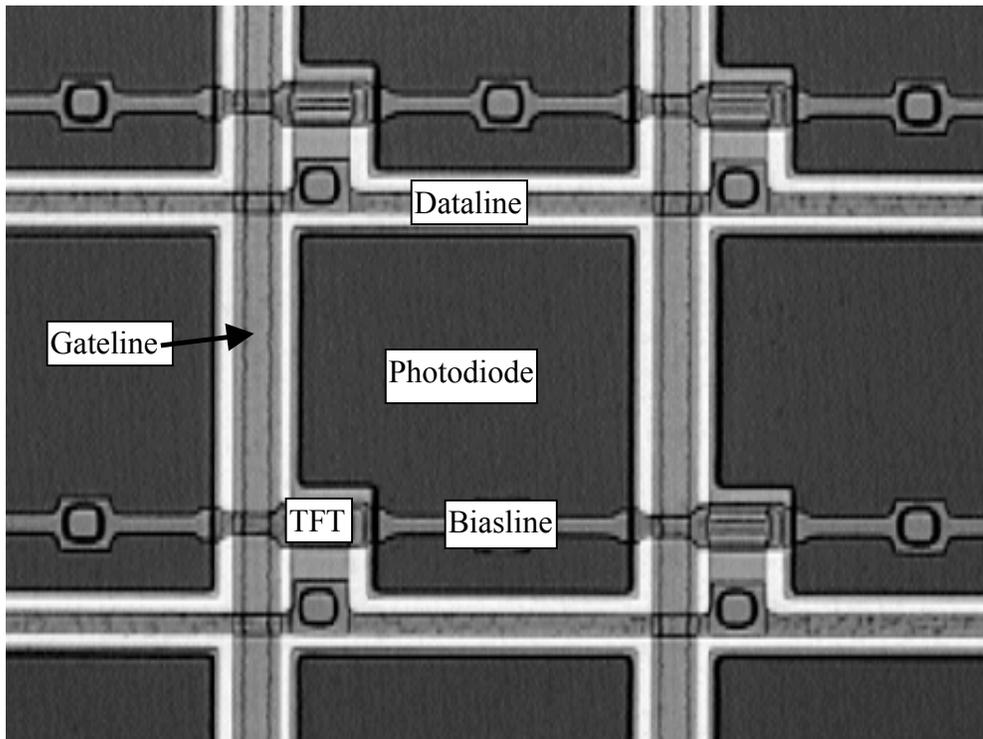
Figure 3: Photomicrograph of a 127 μm pixel.
