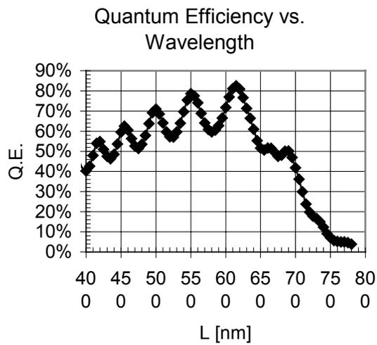
Figure 4. Spectral response of a typical a-Si *nip* photodiode at -5 V reverse bias vs. wavelength.
