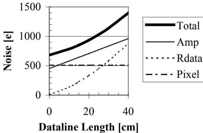
Figure 8: Various contributions of electronic noise associated with pixel size and dataline length. The dashed line is the pixel level noise; the dotted line is the thermal noise generated by the dataline resistance; the fine line is the noise generated by a high quality charge amplifier; and the bold line is the total noise taking these three contributions in quadrature.
