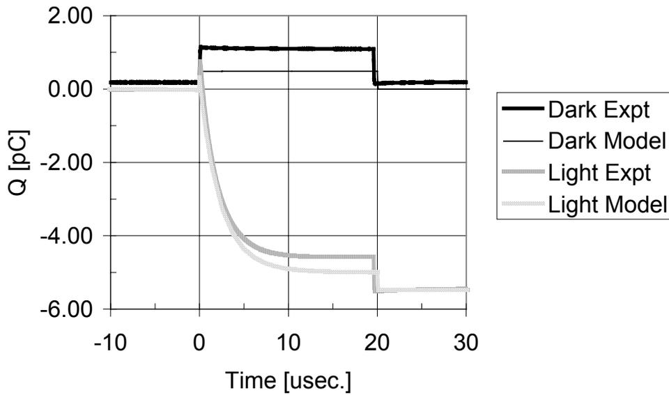
Figure 7: Charge transfer process when gate voltage is changed from  $-8$  to  $+15$  V from  $t=0$  to  $t=20$   $\mu\text{sec}$ . Two cases are shown, one in the dark and one under illumination. Experimental data are compared against Spice modeling for a  $150$   $\mu\text{m}$  pixel.
