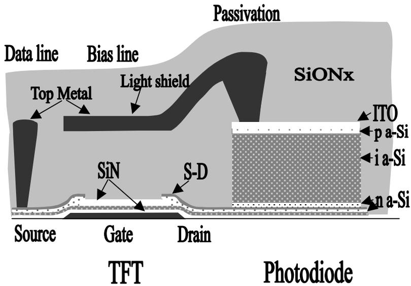
Figure 2: Cross-sectional diagram of a standard pixel in which the photodiode is embedded within the same plane as the TFT and addressing lines.
