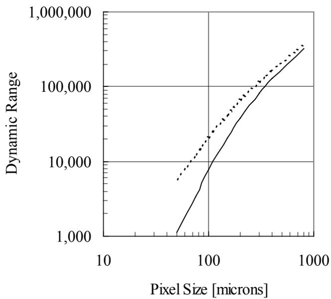
Figure 15: Sensor dynamic range (maximum signal divided by projected electronic noise) vs. pixel size for embedded (solid line) and stacked (dotted line) photodiode architectures.
