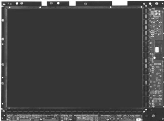
Figure 9: A 30 x 40 cm active area 127  $\mu\text{m}$  pixel image sensor module with gate and data boards TAB bonded to the glass, which is mounted on an aluminum backing plate.
