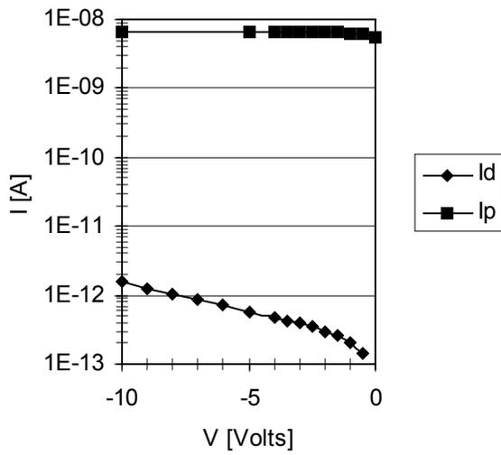
Figure 5: I(V) curve of a 1 mm<sup>2</sup> *nip* photodiode in the dark ( $I_d$ ) and under 570 nm illumination ( $I_p$ ).
