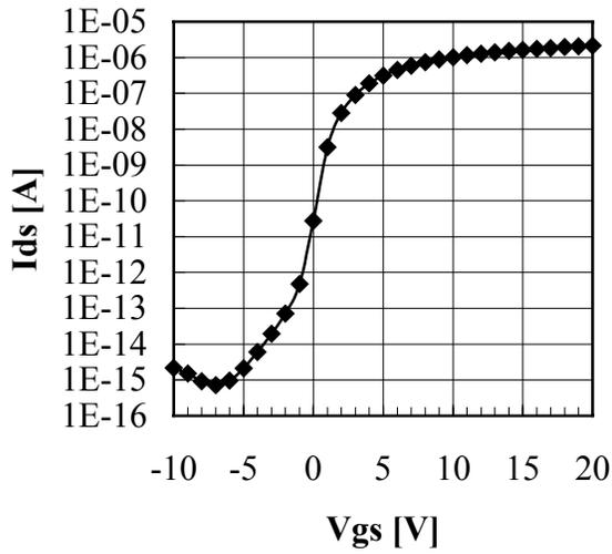
Figure 6: Typical I( $V_{gs}$ ) characteristic of an a-Si TFT at  $V_{ds} = 5$  V, with width  $W = 20\mu\text{m}$  and length  $L = 10\mu\text{m}$  (measured on 500 TFTs in parallel).
