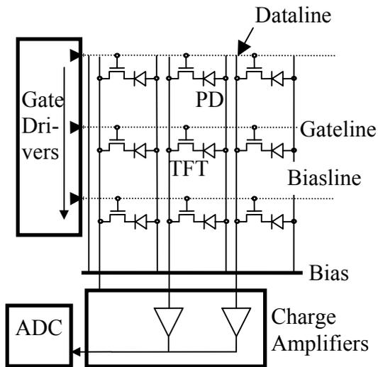
Figure 1: Diagram of TFT/Photodiode array configuration, connected to gate drivers, charge amplifiers, and analog-to-digital converters.
