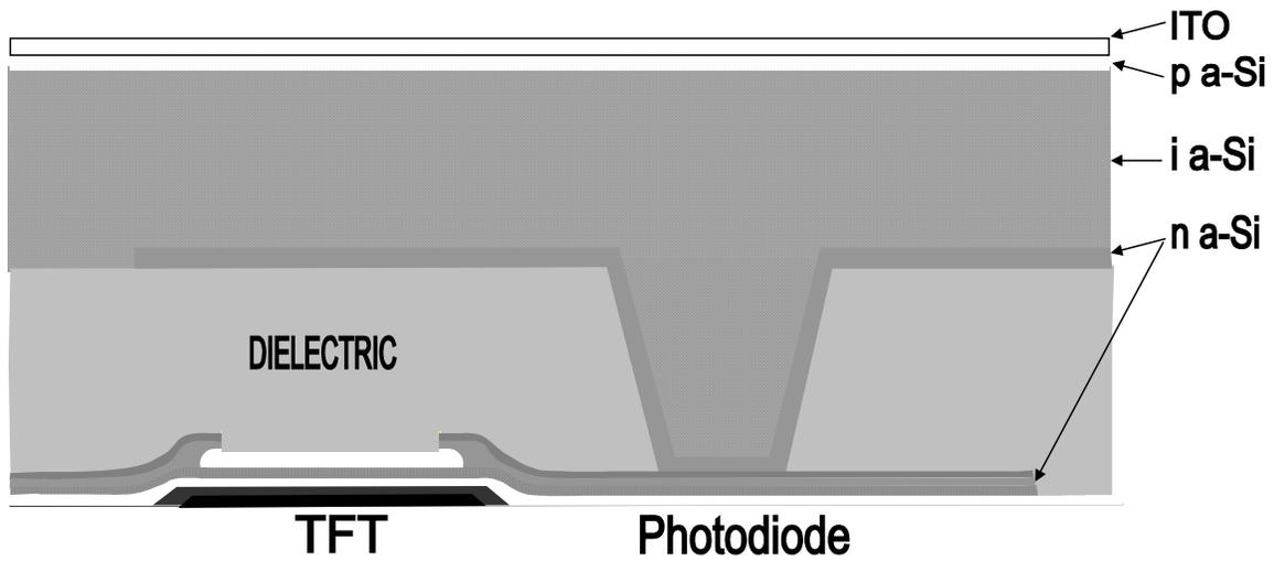
Figure 13: A high fill-factor sensor architecture in which the photodiode is stacked on top of the TFT and addressing lines.
