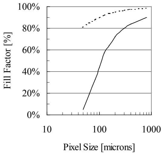
Figure 14: Sensor fill factor vs. pixel size for embedded (solid line) and stacked (dotted line) photodiode architectures.
