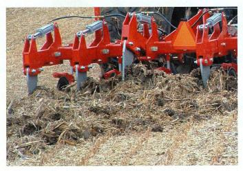
Automatic bump and run hydraulic trip system provides on the go stone protection. Accumulator system can be readily charged to match soil conditions. Spring loaded 20" serrated coulters cut surface stalks and enhance flow of residue.
