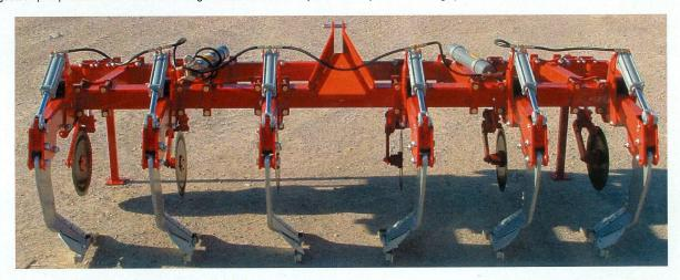
The Howard Paratill leg was uniquely designed to restructure the soil through vertical and diagonal forces. The leg lifts the soil and while in motion the offset design provides a diagonal sheering effect. The result, a more complete restructuring of the whole area. This provides for better root penetration, enhanced nutrient flow and plant development.
