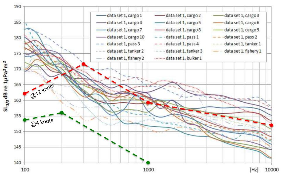
Source levels of 20 vessels of different type at a shipping route close to Rotterdam. (SONIC D2.5, 2015), TNO
