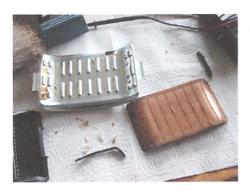
Velcro; To separate the plates I cut 1/16" wide strips of the loop section of self adhesive Velcro and stuck them on the steel plate where the old adhesive had been. See picture 4.
