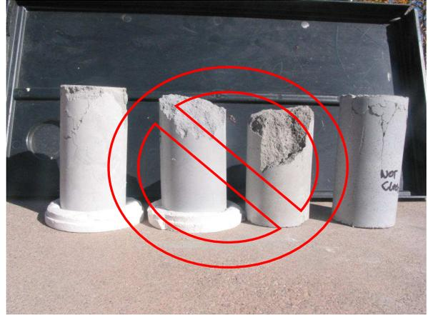
**Figure 2: Incorrect cylinder breaks**
