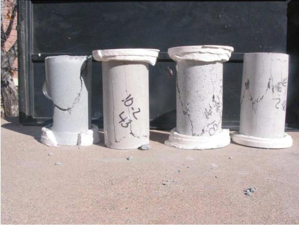
**Figure 1: Correct cylinder breaks**
