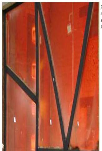
GUENIS Products *INTERFLAM* and *INTERFIRE* offer a combination of fire protection and excellent safety characteristics with a fire resistance time up to 120 minutes. Benefits include:
