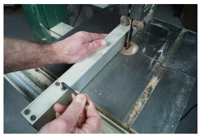
Set your bandsaw fence to the line you traced on the table.
