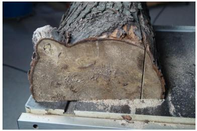
Snap another line and make a second cut perpendicular to the first. This will make it much easier to keep the half round against the fence.
