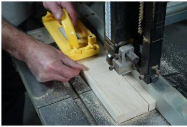
Make a test cut. If the board feeds perfectly, the fence is fine. If the outfeed end of the board trails away from the fence and a gap opens between the board and fence, the fence angle is too "open," the outfeed end of the fence too far to the left. If the board binds as you're cutting it the fence is pinching, the outfeed end is too far to the right. Adjust the fence as needed. It's not uncommon to have to do this test a couple times to tweak the fence into just the right position.
