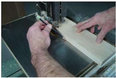
Trace the edge of the board onto the bandsaw table. You have experientially found the drift of the blade, and are now transferring the drift angle to the saw.
