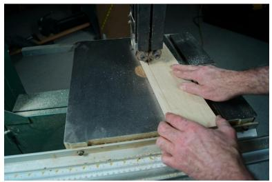
Freehand follow the line, carefully adjusting your feed as needed in order to cut dead straight. Once you feel you're feeding at the correct angle to cut straight, freeze the board in place and shut off the saw.
