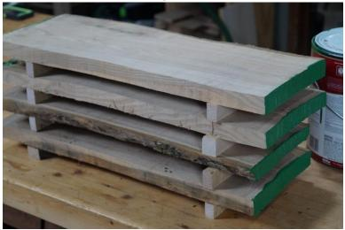
Seal the ends of the boards (latex paint works fine) and stack the boards with stickers between each layer for uniform air flow. Be sure the stickers are aligned with each other vertically. In order to prevent stains from the stickers, it's a good idea to cut them from the same material you're drying.
