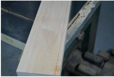
Using a board with a perfectly straight (jointed) edge, make a line parallel to the edge. Use a board that's approximately 14" long.
