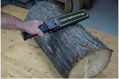
Run the metal detector over all sides of the log to make sure it's clean.
