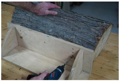
Screw the sled to the log. Two fasteners, in the approximate center of the log, will do it. As time goes on you may have to add holes to your sled in order to have holes that align with the log's center. Don't worry about the screw holes in the log. There will always be slab wood from the log exterior that you won't use.
