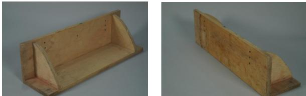
A log can roll, dangerously, during the cut, unless you stabilize it. This simple sled acts as an outrigger to keep the log stable. 3/4" plywood works well. Make the base and the vertical 6" wide. Make it as long as the log you're going to cut. Drill a few holes for lag screws.
