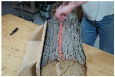
Hook a chalk line in the end of the log you notched, and visually align the other end with the pith of the log. Snap a line.
