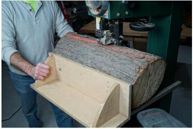
Cut the log into two halves, freehand following the snap line. Be sure to set up outfeed support. Logs are heavy! If there's any question about being able to make the cut, get help. Cut as straight as you can. The better the first cut is, the more lumber you'll get out of your log.
