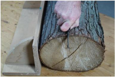
Using a knife, make a V in the log that aligns with the center of the "bullseye," the pith of the log. We'll take advantage of the V notch to snap our line.
