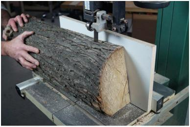
Add a tall fence as needed to fully support your log. Set the distance from the face of the fence to the bandsaw blade based on the thickness of the lumber you want to produce. Remember the lumber will shrink as it dries, and eventually you'll be planing off bandsaw marks, so allow enough thickness to compensate.
