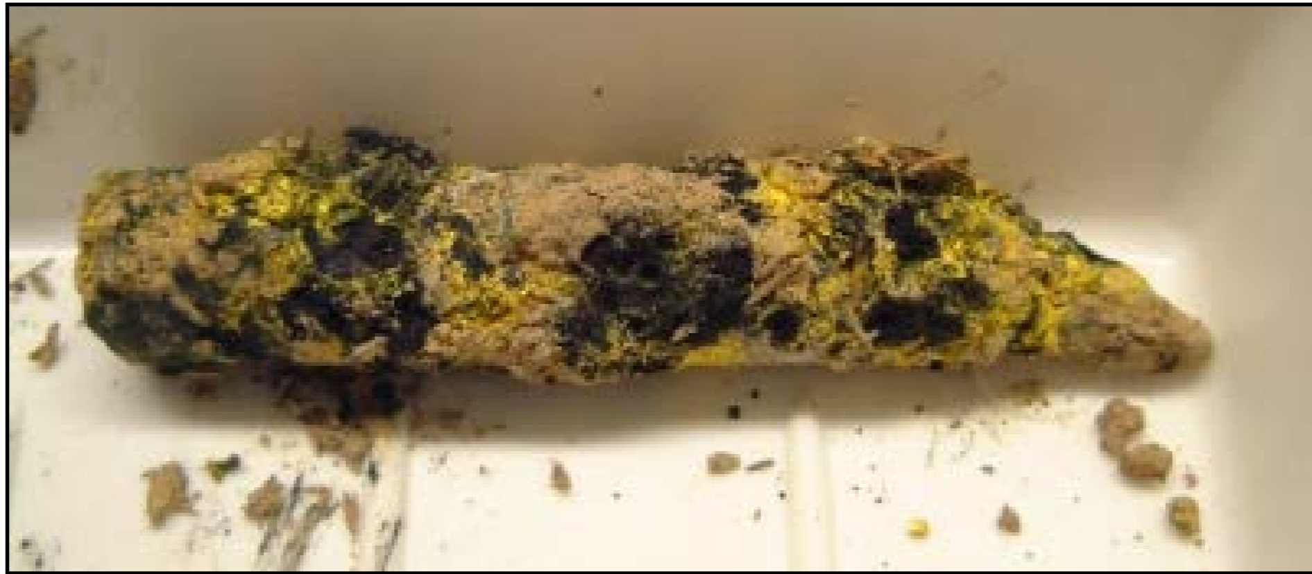
Armor-piercing DU penetrator after three years in natural environment
