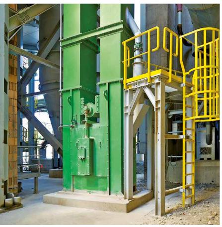
Elevator boot with parallel tensioning device
