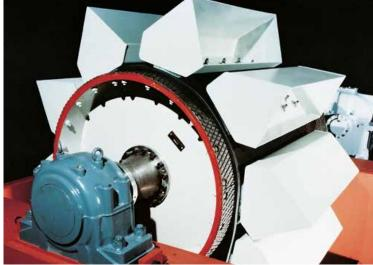
Drive drum with friction lining
