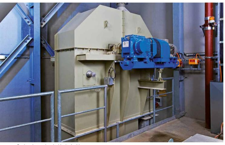
Bucket elevator head with single drive
