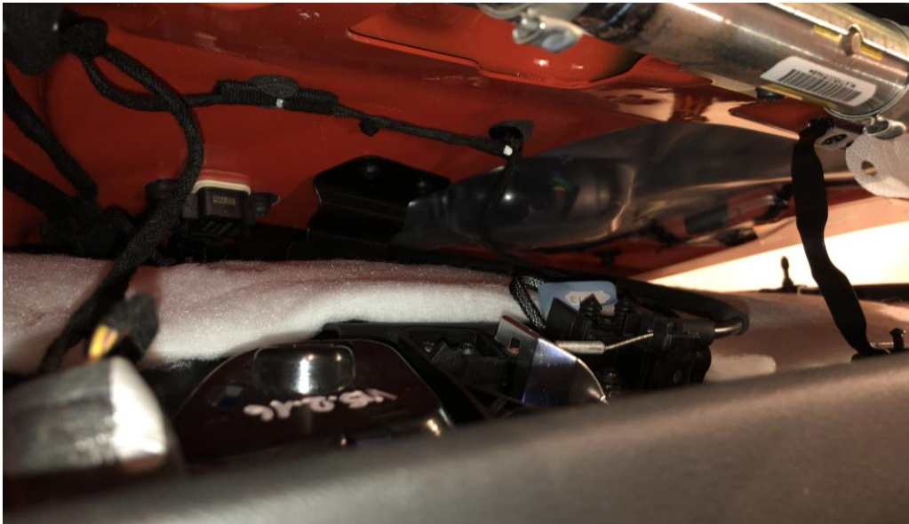
Backside of door trim showing multiple electrical and mechanical connectors and tethers
