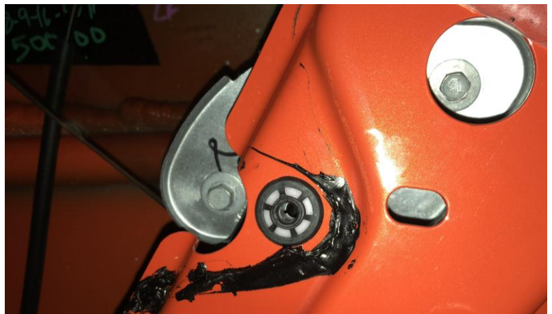
Window aligned to allow access to regulator bolts
