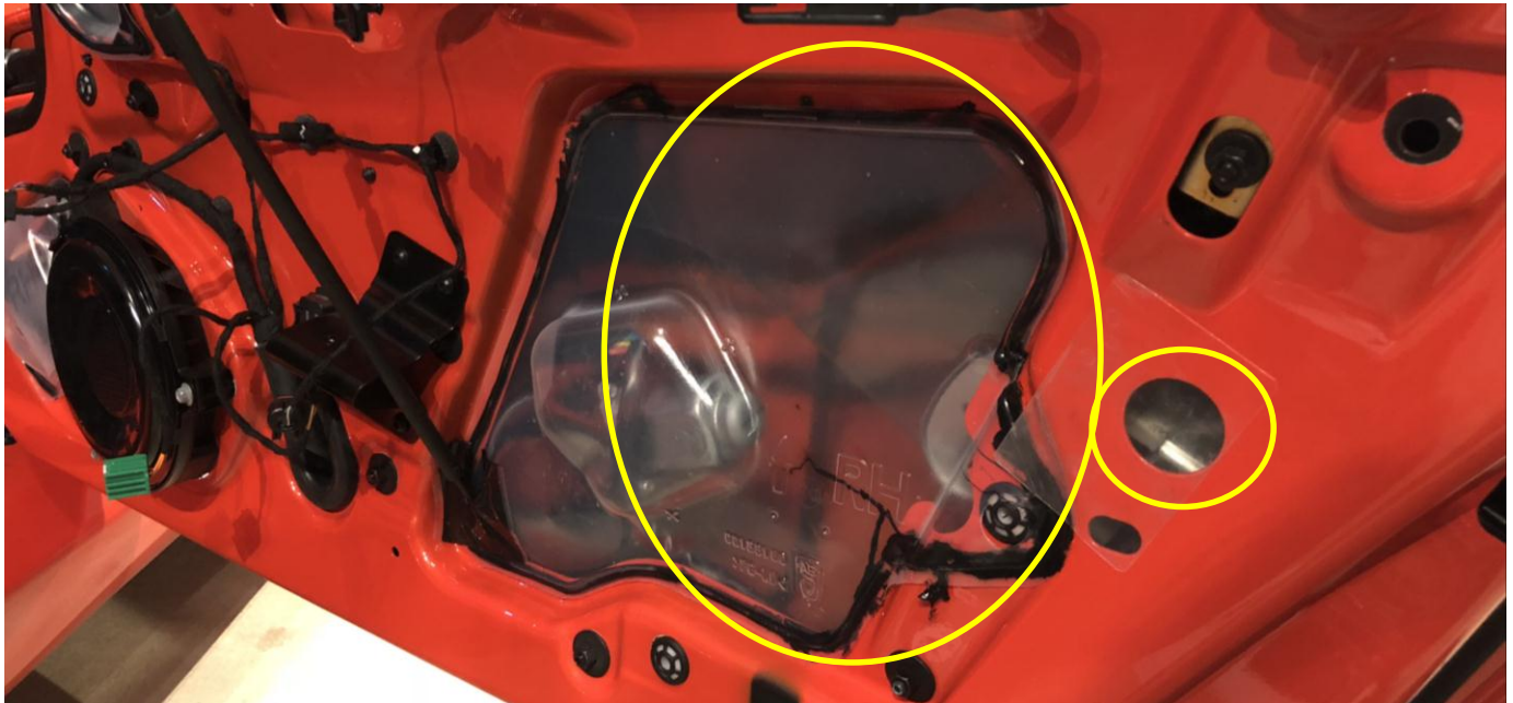
Peel back vapor barrier shown to allow access to window/regulator bolts
