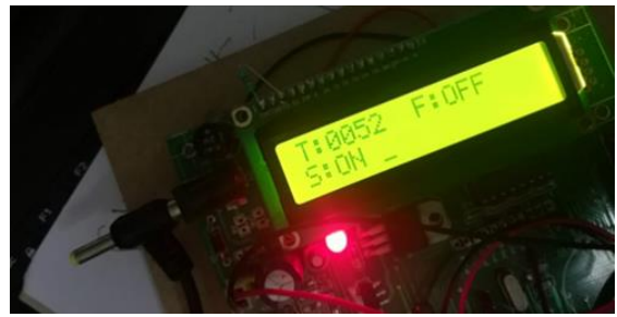
Fig.3.2. Temperature and smoke measured time.
